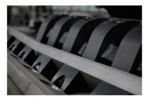
GE series adopts a special rotor design and it is an economical crusher. The width of the rotor ranges from 500mm to 1400mm. The rotor adopts high-efficiency scissor cutting technology, the welded cavity of the entire steel structure is combined with the V-shaped rotor to ensure stable machine operation and reliable performance. The compact body design facilitates cavity maintenance, quick cleaning and replacement of rotary knives, fixed knives and screens.
